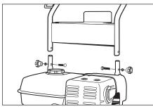
**Step 1** Attach the handle to the frame of the pressure washer. Align holes, insert bolt, and tighten with knob.
